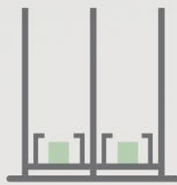
Warm-edge spacer reduces condensation
